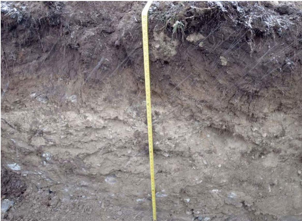
**Figure 7-19: Soil Profile from Test Pit**
